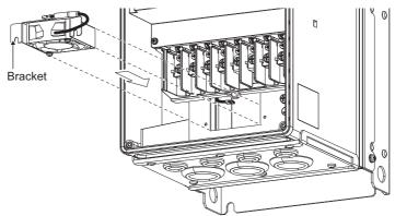
(3) Reconnect the fan connector, and then place the connector case from the above.
