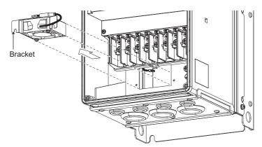
(5) Remove the installation screws, and then remove the fan.
