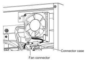
(3) Remove the installation screws, and then remove the bracket.
