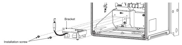
(4) Remove the installation screws, and then remove the fan.
