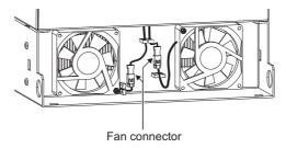
(3) Attach the fan cover with the installation screws. (tightening torque 1.4 to 1.9 N•m)
