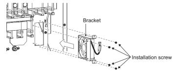
(3) Reconnect the fan connector, and then place the connector case from the above.
