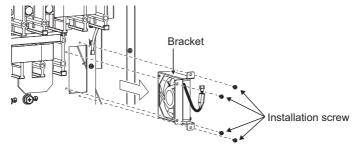
(4) Remove the installation screws, and then remove the fan.
