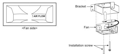
(2) Attach the bracket to the inverter.
