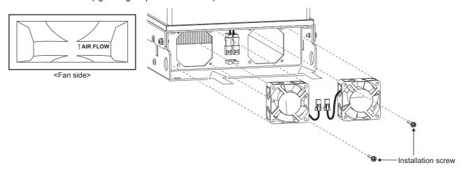
(2) Route the fan lead through the clamp, and then reconnect the fan connectors.
