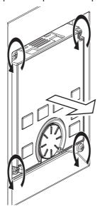
• To reinstall the operation panel, align its connector on the back with the PU connector of the inverter, and insert the operation panel. After confirming that the operation panel is fit securely, tighten the screws in the diagonal order. (Tightening torque: 0.39 to 0.49 N·m)
