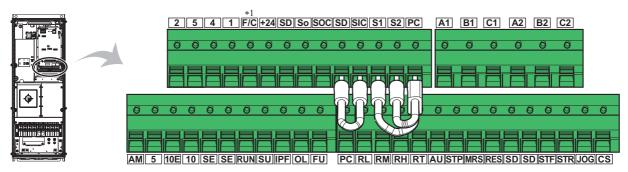
\*1 This terminal operates as terminal FM for the FM type, and as terminal CA for the CA type.
