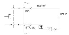
External signal input using transistor (source logic)
