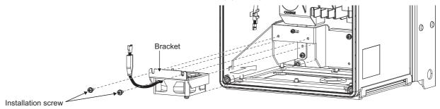
(3) Reconnect the fan connector, and then place the connector case from the above.
