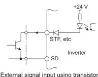
External signal input using transistor (sink logic)
