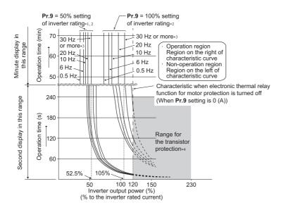
This function detects the overload of the motor, stops the operation of the inverter's output transistor, and stops the output. (The operation characteristic is shown on the left.)
