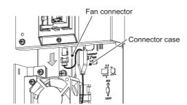
(3) Remove the installation screws and the bracket, and then remove the fan.
