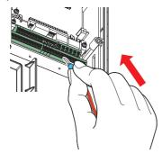
When using a single wire or stranded wires without a crimp terminal, push the open/close button all the way down with a flathead screwdriver, and insert the wire.
