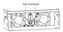
(3) Remove the installation screws, and then remove the fan.
