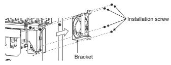
(4) Remove the installation screws, and then remove the fan.
