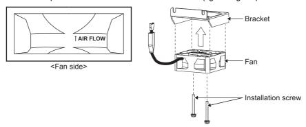
(2) Fix the bracket to the inverter with the installation screws. (tightening torque 1.4 to 1.9 N•m)
