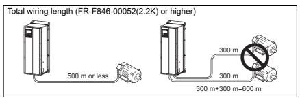
When driving a 400 V class motor by the inverter, surge voltages attributable to the wiring constants may occur at the motor terminals, deteriorating the insulation of the motor. In this case, take one of the following measures.
