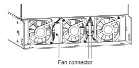
(3) Attach the fan cover with the installation screws. (tightening torque 1.4 to 1.9 N•m)
